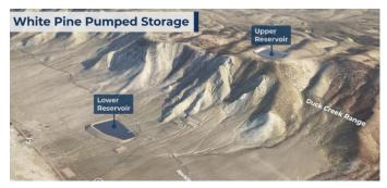
The White Pine Pumped Storage project is the second rPlus Hydro project to reach the final application license milestone this year, and is one of only a handful of pumped storage projects to reach this stage in the past two decades. The project will provide Nevada with significant energy storage capability. Source: rPlus Hydro
