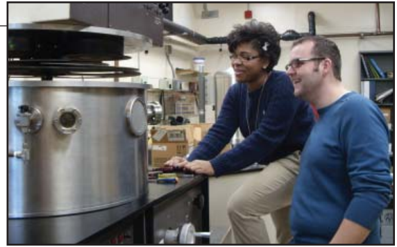
Miami University's Lyndsey McMillon and her mentor, Jeremiah McNatt, a NASA electrical engineer, are opening the Sputter Machine to retrieve the deposited thin film solar cells which will then be characterized by a series of additional tests and analysis, including, X-ray diffraction, spectrophotometry, thickness measurement, and Hall resistivity measurement. Photo: NASA's Undergraduate Student Research Program.
